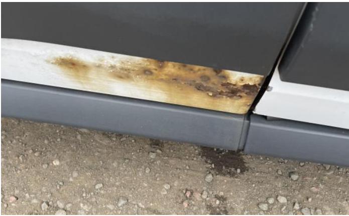
3: Wing osf Rusted Over 5mm
