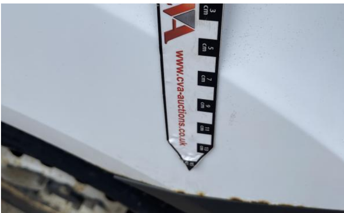
5: Qtr Panel osr Rusted Over 5mm
