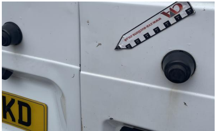
6: Door osf Rusted Over 5mm
