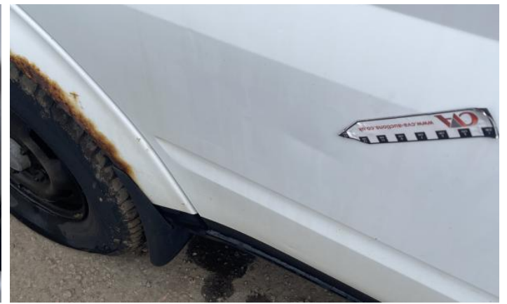
10: Door nsr Dented With Paint Damage
