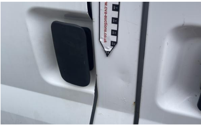
9: Qtr Panel nsr Rusted Over 5mm
