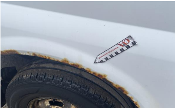
5: Wing osf Rusted Over 5mm
