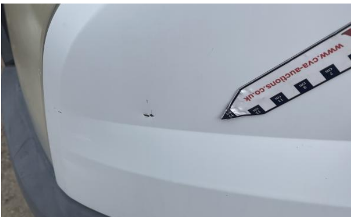
11: B Post ns Rusted Over 5mm
