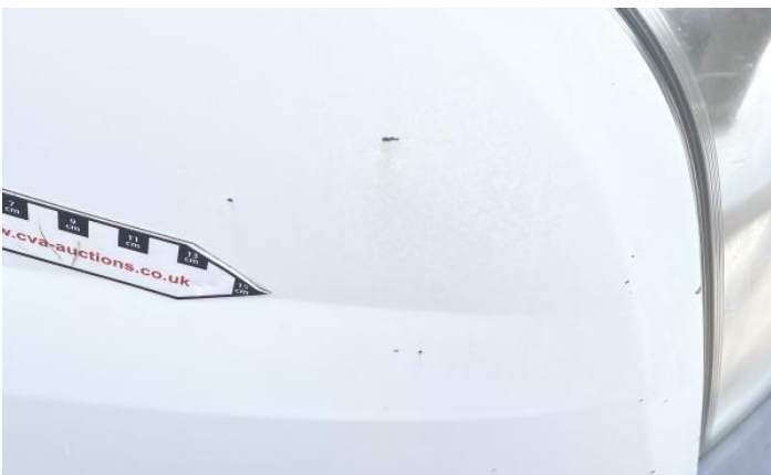
5: Roof Rusted Over 5mm
