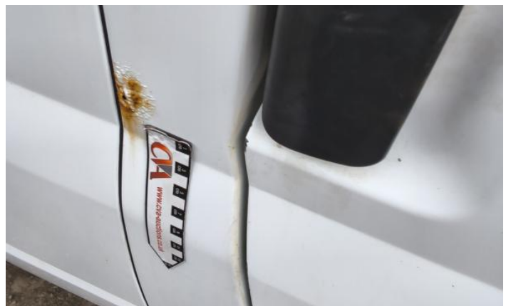
6: Wing osf Rusted Over 5mm
