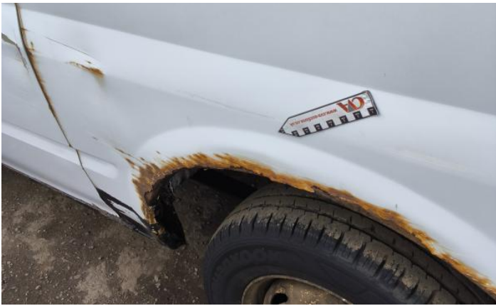
9: Qtr Panel osr Rusted Over 5mm
