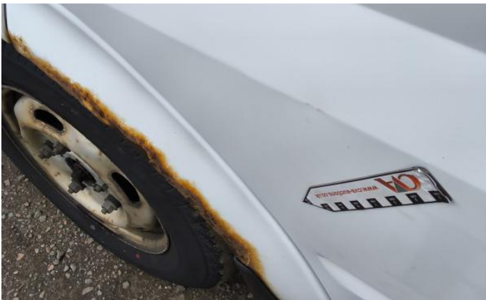
11: Qtr Panel nsr Dented With Paint Damage
