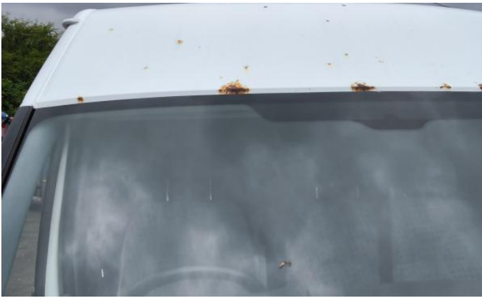
3: Sill os Rusted Over 5mm
