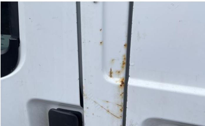
11: Qtr Panel nsr Rusted Over 5mm
