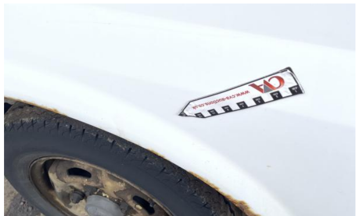
6: Sill os Rusted Over 5mm
