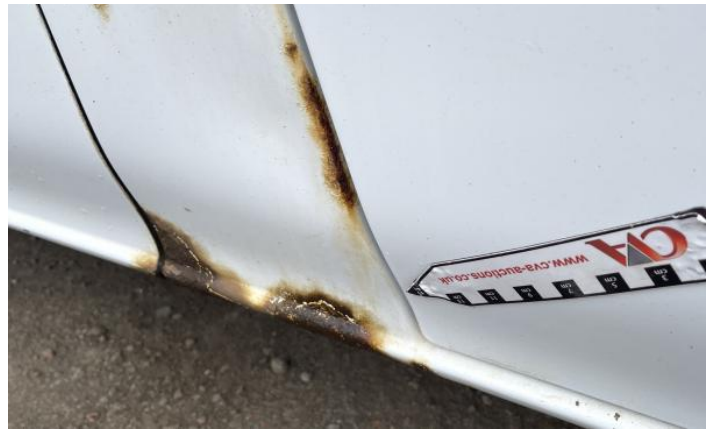
4: Wing osf Rusted Over 5mm
