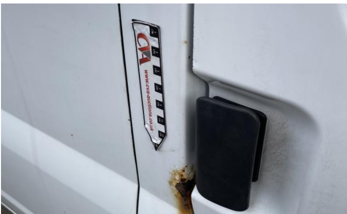
5: Door osf Rusted Over 5mm
