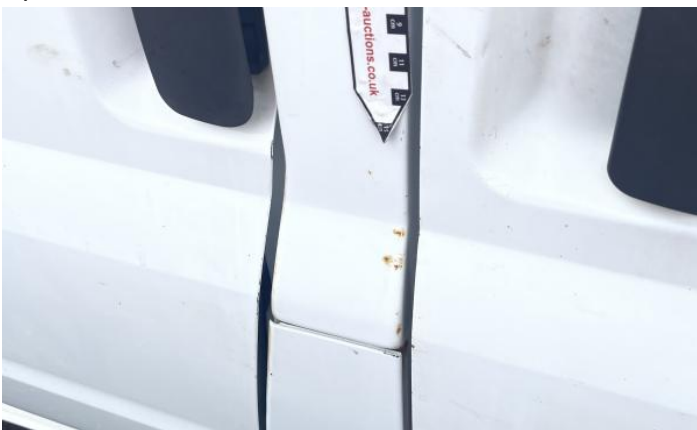
11: Door nsr Rusted Up To 5mm
