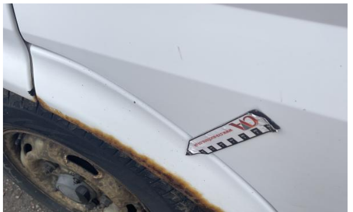
12: Sill ns Rusted Over 5mm
