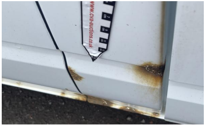
4: Wing osf Rusted Over 5mm
