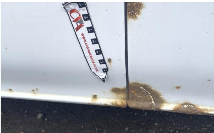
5: Door osf Rusted Over 5mm
