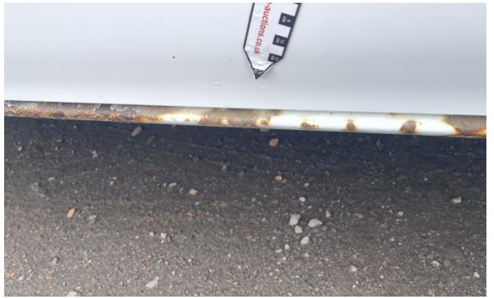
10: Qtr Panel nsr Dented With Paint Damage
