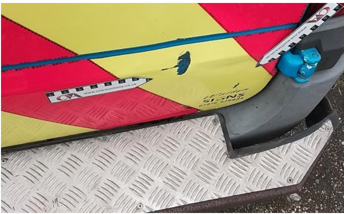
15: Door osr Dented Over 30mm
