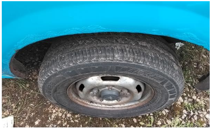
10: Qtr Panel nsr Dented Over 30mm
