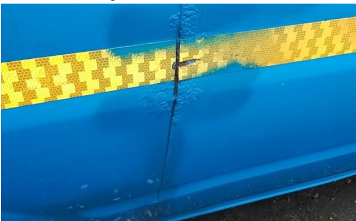
17: Door osr Dented With Paint Damage
