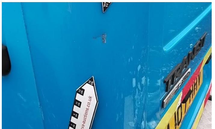
12: Qtr Panel nsr Rusted Over 5mm
