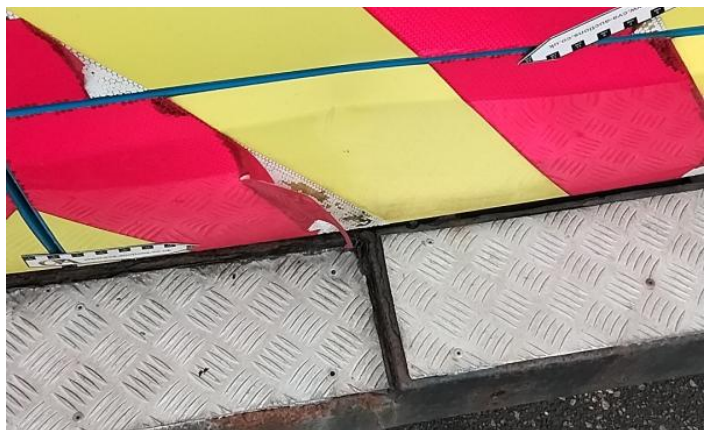
12: Qtr Panel Moulding ns Scuffed (Unpainted) Over 100mm
