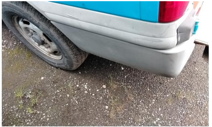
10: Qtr Panel nsr Rusted Over 5mm
