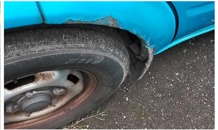
4: Wing nsf Scratched Over 25mm Thru Paint
