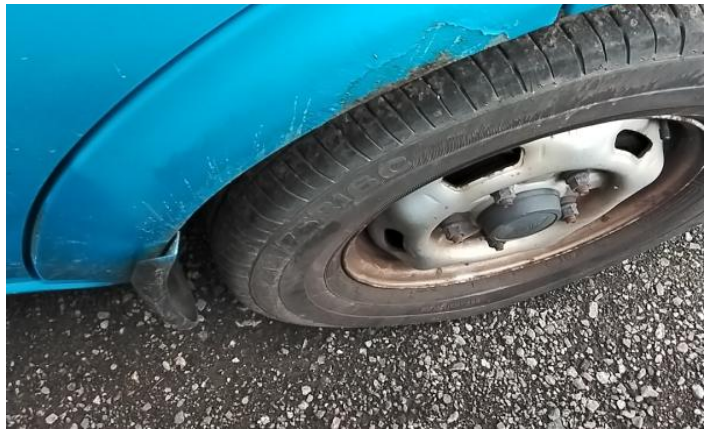
16: Qtr Panel osr Rusted Over 5mm
