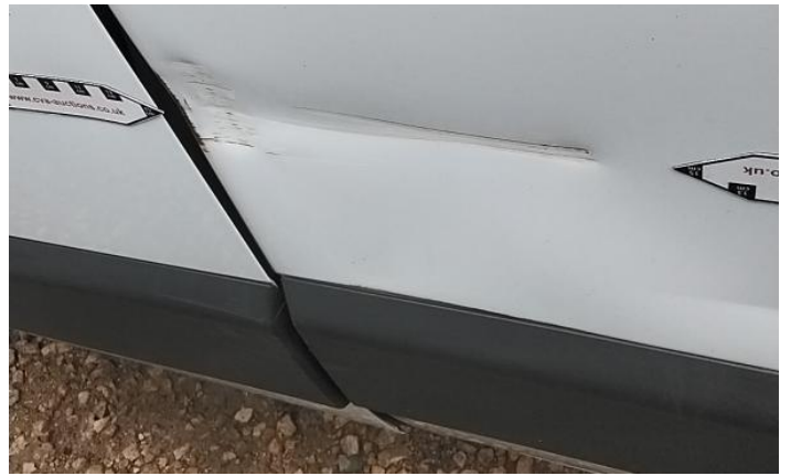
16: Qtr Panel nsr Dented Over 30mm
