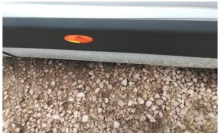
18: Qtr Panel nsr Dented With Paint Damage
