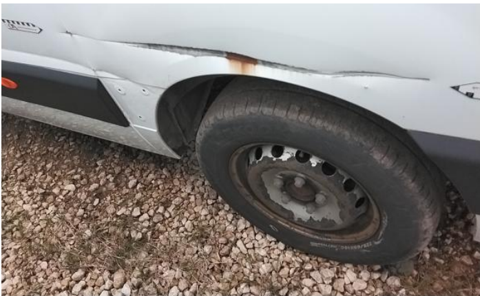
23: Qtr Panel nsr Dented With Paint Damage
