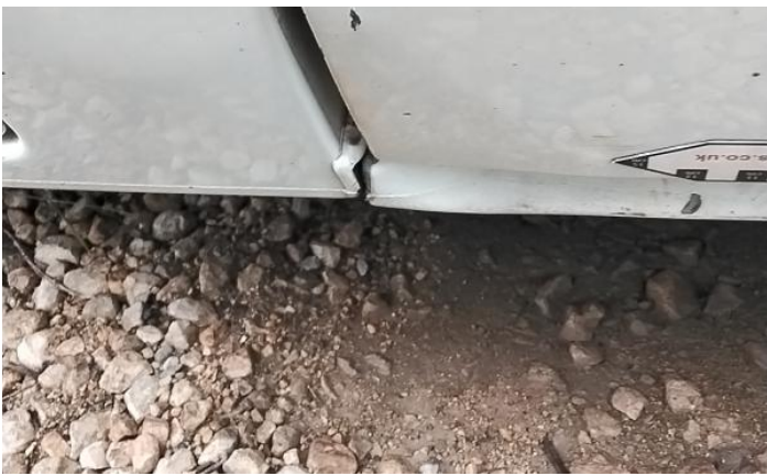
9: Sill ns Dented Over 30% Of Panel
