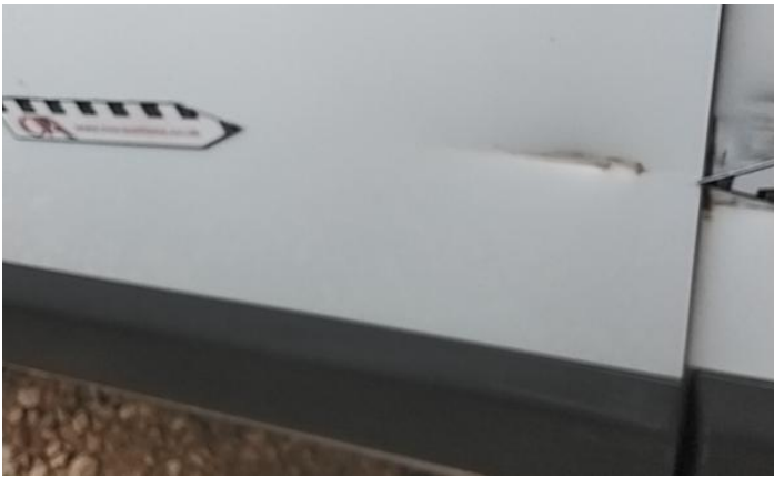
15: Qtr Panel nsr Dented With Paint Damage
