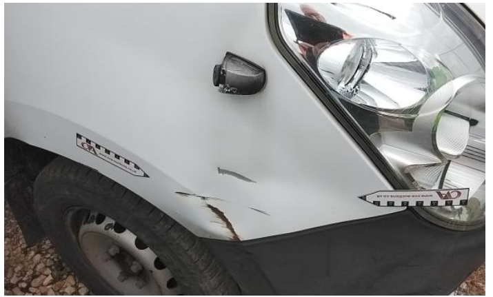
34: Qtr Panel osr Dented With Paint Damage
