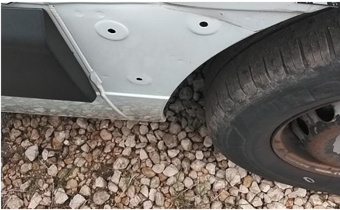
21: Qtr Panel nsr Dented With Paint Damage
