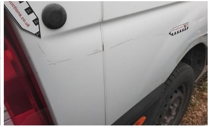
28: Door nsr Dented Over 30% Of Panel
