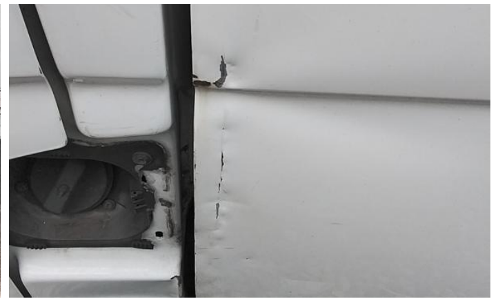
10: B Post ns Dented Over 30mm
