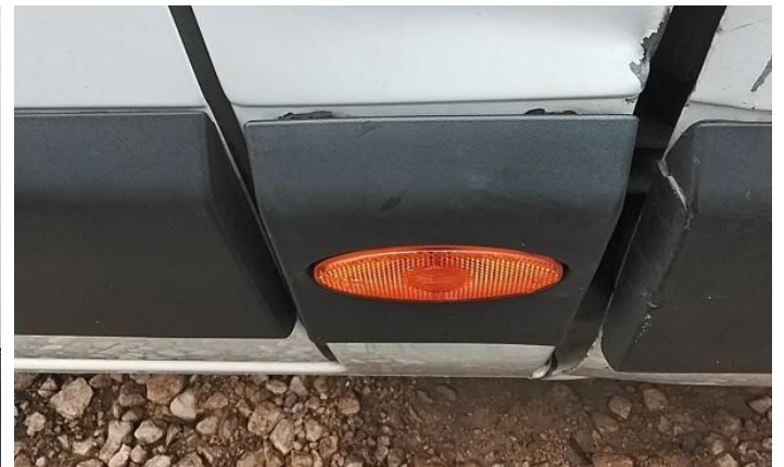
6: Door Moulding nsf Scuffed (Unpainted) Over 100mm
