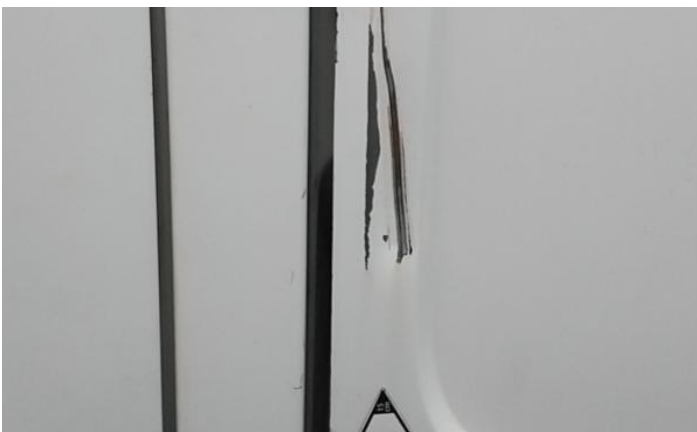
11: Qtr Panel nsr Dented Over 30mm
