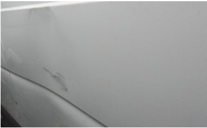
33: Qtr Panel osr Dented With Paint Damage
