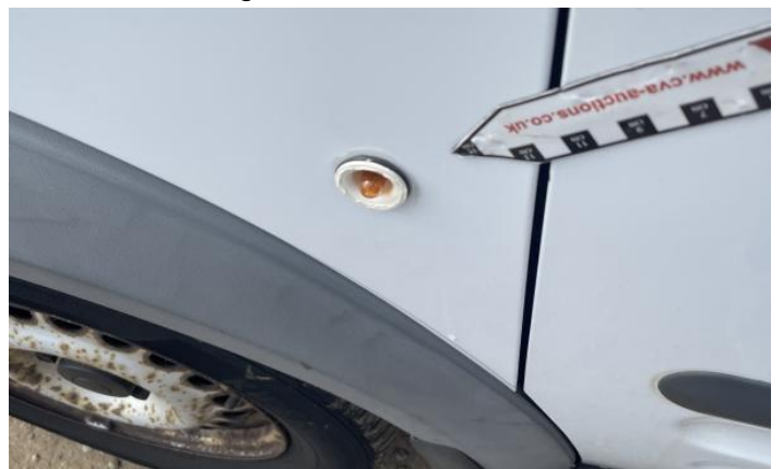
6: Qtr Panel nsr Dented With Paint Damage
