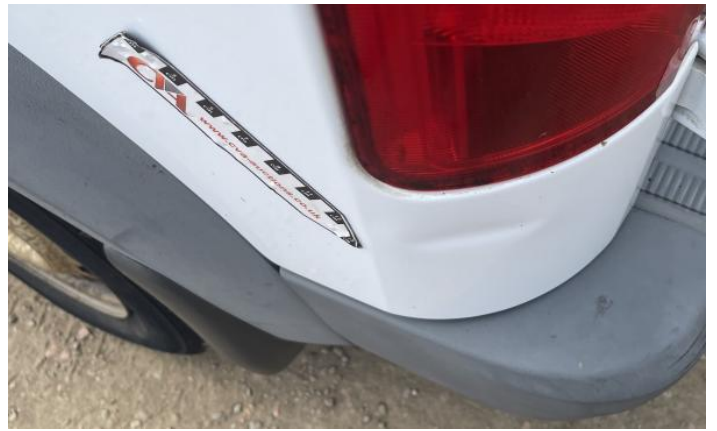
4: Qtr Panel osr Dented With Paint Damage
