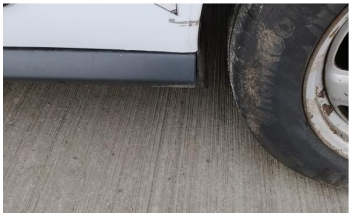
6: Wing nsf Poor Previous Repair Poor Colour
