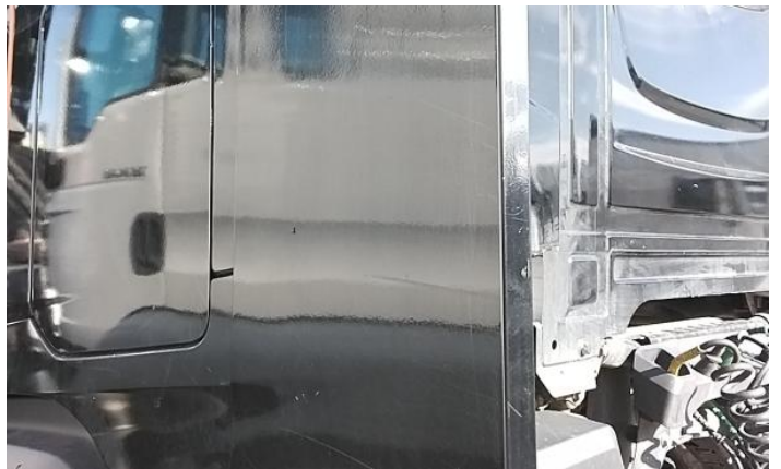
6: Door nsf Dented With Paint Damage
