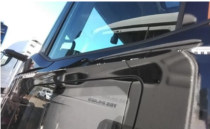
5: Door nsf Dented With Paint Damage
