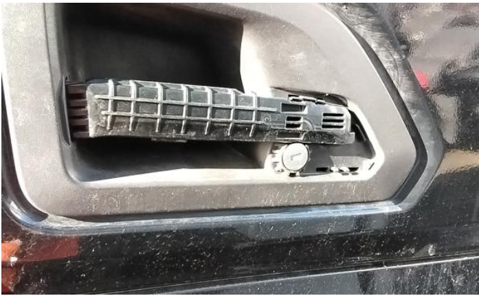
9: Qtr Panel Moulding ns Broken Replace
