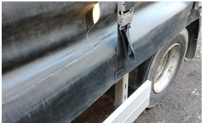
6: Door nsf Scratched Over 25mm Thru Paint
