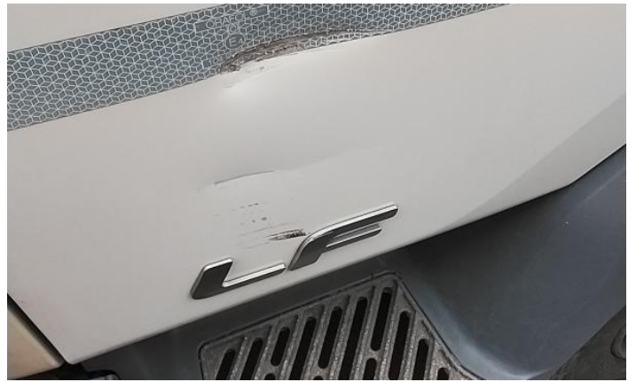
4: Bumper Front Scratched Over 100mm Thru Paint
