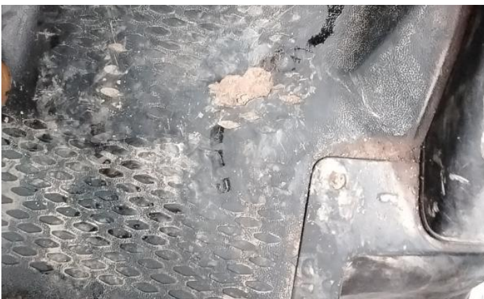
11: Screen Front Chipped Over 10mm
