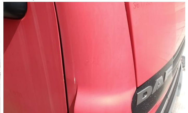
12: Door osf Dented Over 2 UpTo 10mm
