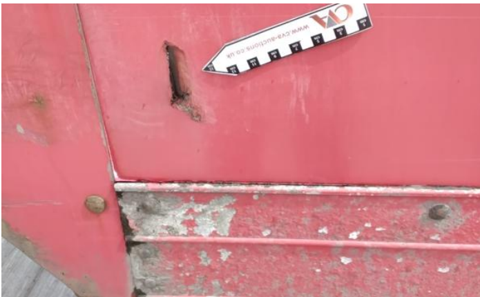
5: Door Moulding nsf Scratched (Painted) Over 25mm Thru Paint
