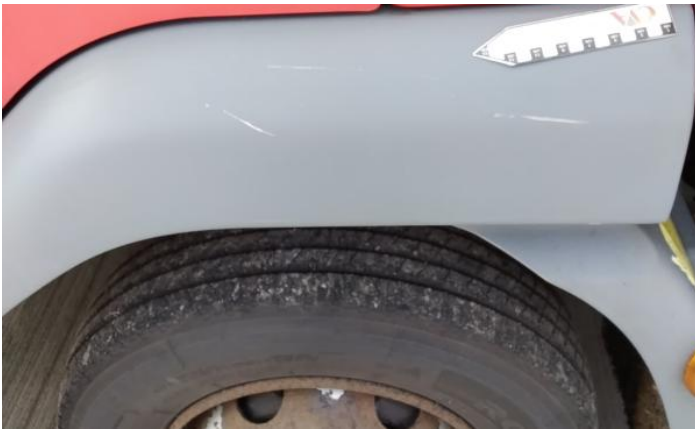
3: Moulding nsf Wing Broken Replace
