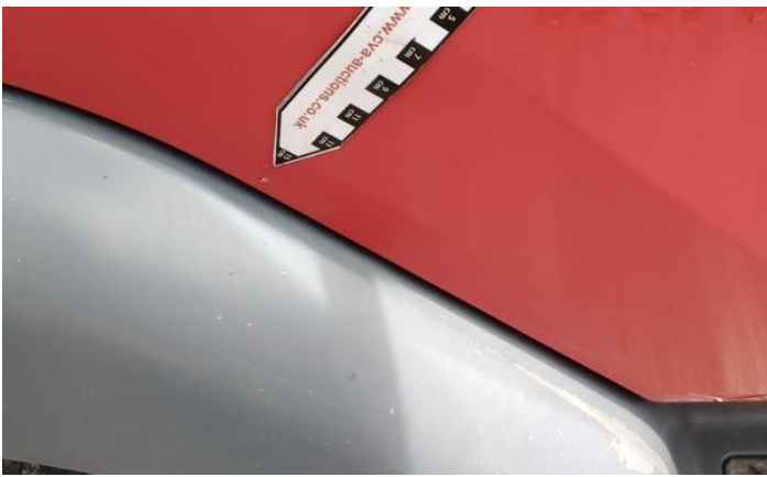
9: Door osf Scratched Over 25mm Thru Paint
