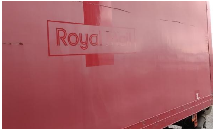
4: Door nsf Scratched Over 25mm Not Thru Paint
