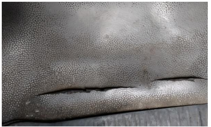
10: Moulding osf Wing Scratched (Painted) Over 25mm Thru Paint
