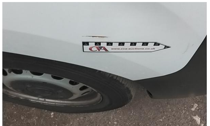
6: Door osf Scratched Over 25mm Thru Paint
