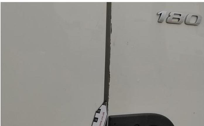
11: Wing Front Arch Extension os Scuffed (Unpainted) Over 100mm
