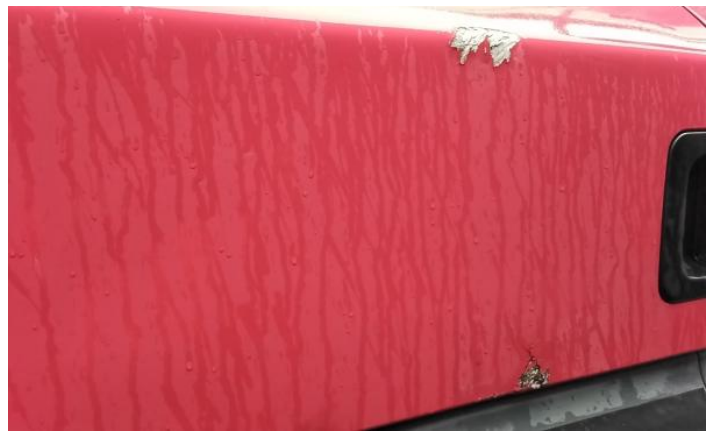
4: Panel Front Scratched Over 25mm Thru Paint
