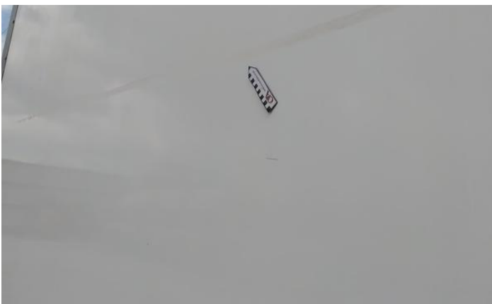
5: Wing nsf Scratched Over 25mm Thru Paint
