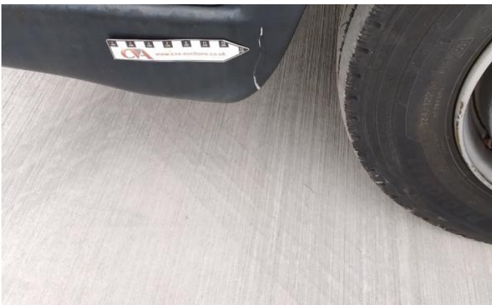
3: Bumper Front Cracked Over 25mm
