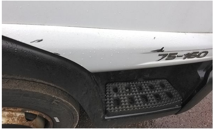
4: Door nsf Dented With Paint Damage
