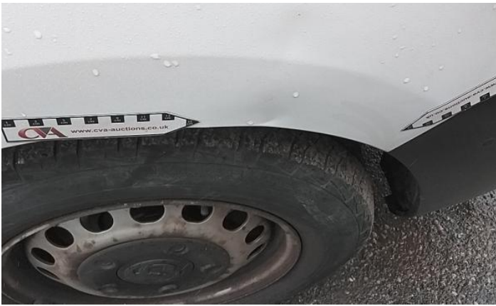
3: Qtr Panel nsr Dented With Paint Damage
