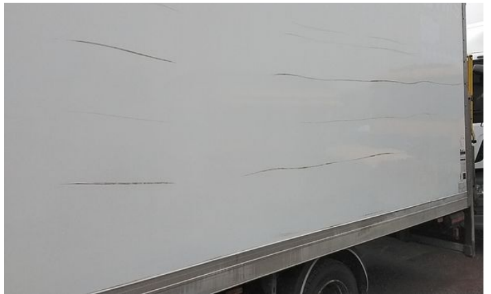
4: Panel Front Scratched Over 25mm Thru Paint
