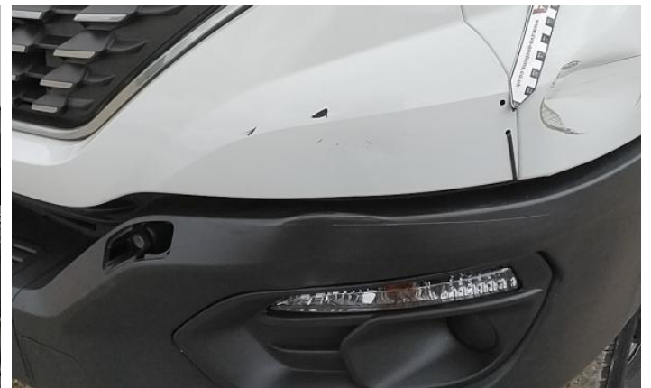
6: Bumper Front Dented Over 30mm
