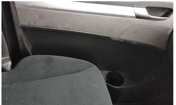
6: Door osf Scratched Over 25mm Thru Paint
