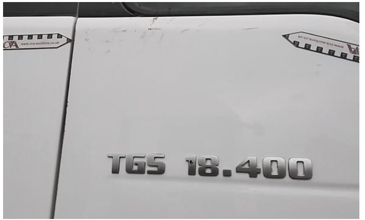
4: Wing nsf Scratched Over 25mm Thru Paint
