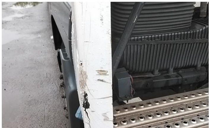
4: Qtr Panel nsr Dented With Paint Damage
