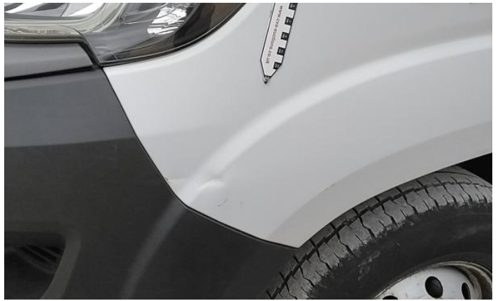
4: Bumper Front Moulding Scuffed (Unpainted) Over 100mm
