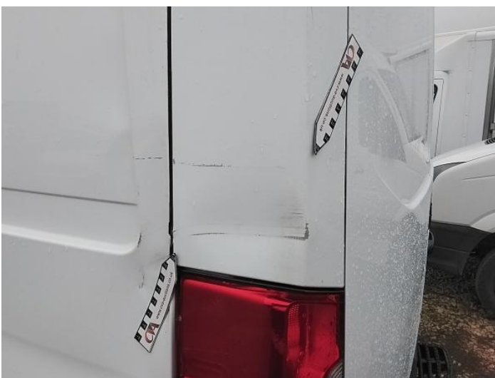
13: C Post ns Dented Over 30mm
