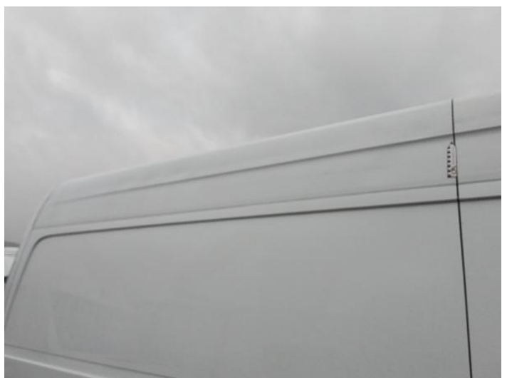
20: Qtr Panel osr Dented Over 30mm
