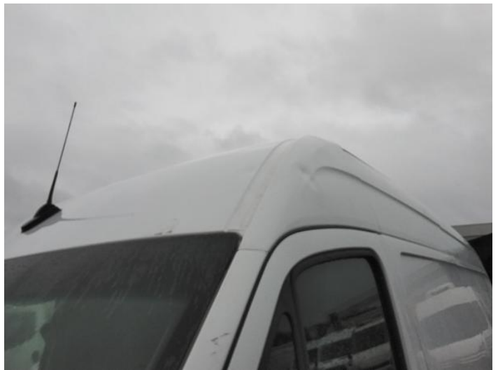
6: Roof Dented Over 30mm
