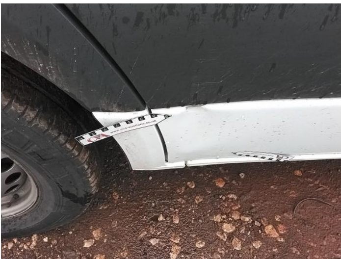
7: Door nsf Dented Over 30mm
