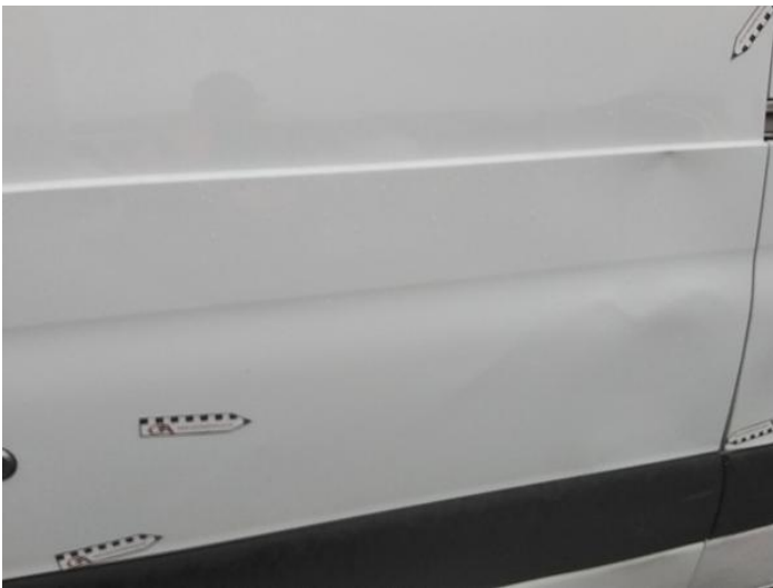
5: Qtr Panel nsr Dented Over 30mm
