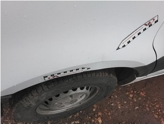
3: Wing nsf Dented Over 30mm
