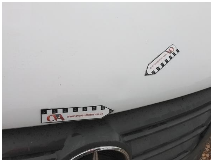
2: Bonnet Dented Over 30mm
