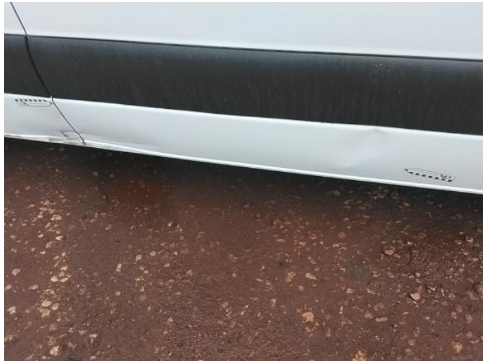
24: Qtr Panel osr Dented Over 30mm
