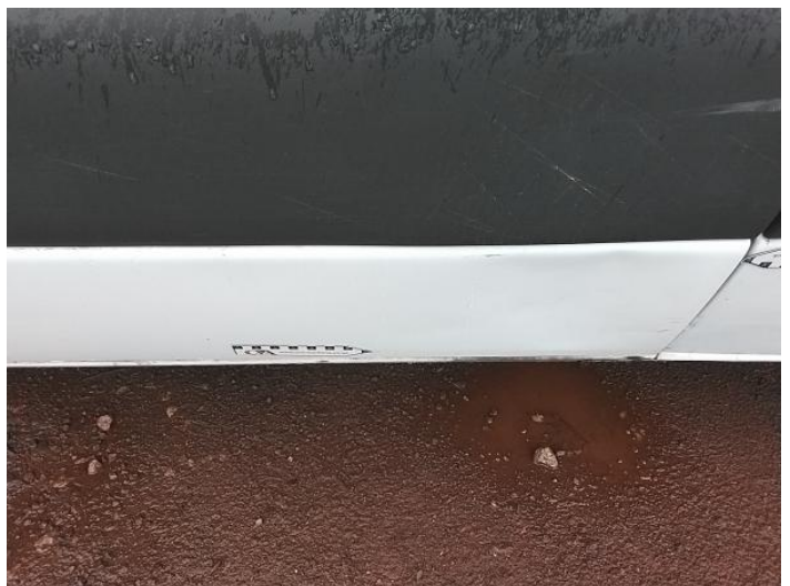
8: Qtr Panel nsr Dented Over 30mm
