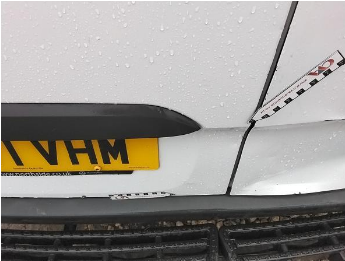
15: Door nsr Dented Over 30mm
