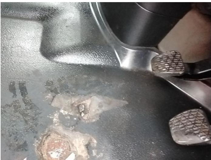
25: Carpets Front Holed Over 3mm
