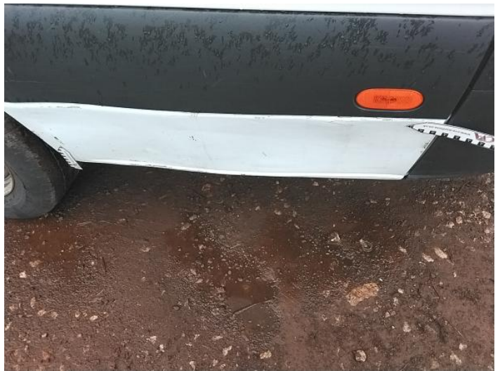
12: Qtr Panel nsr Dented Over 30mm
