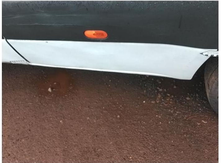
10: Qtr Panel nsr Dented Over 30mm
