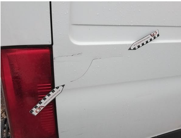
17: Qtr Panel osr Dented Over 30mm
