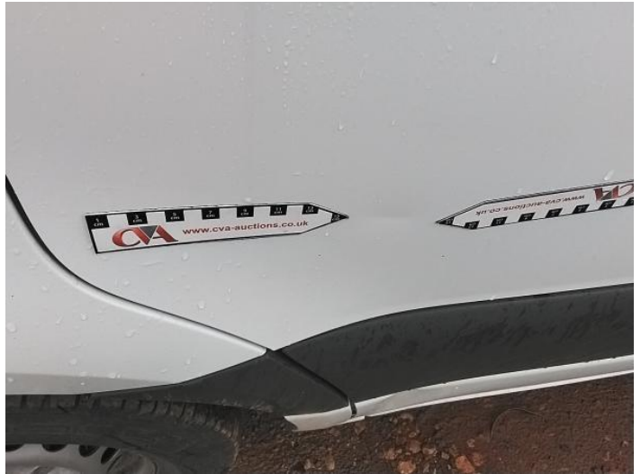
4: Door nsf Dented Over 30mm
