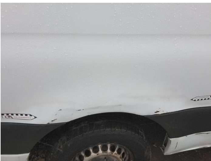
19: Qtr Panel osr Dented Over 30mm
