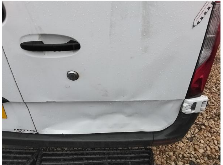
16: Door osr Dented Over 30mm
