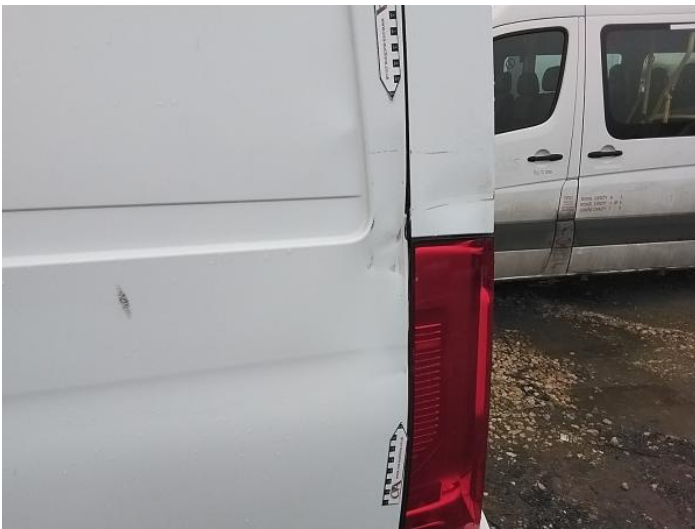
11: Qtr Panel nsr Dented Over 30mm
