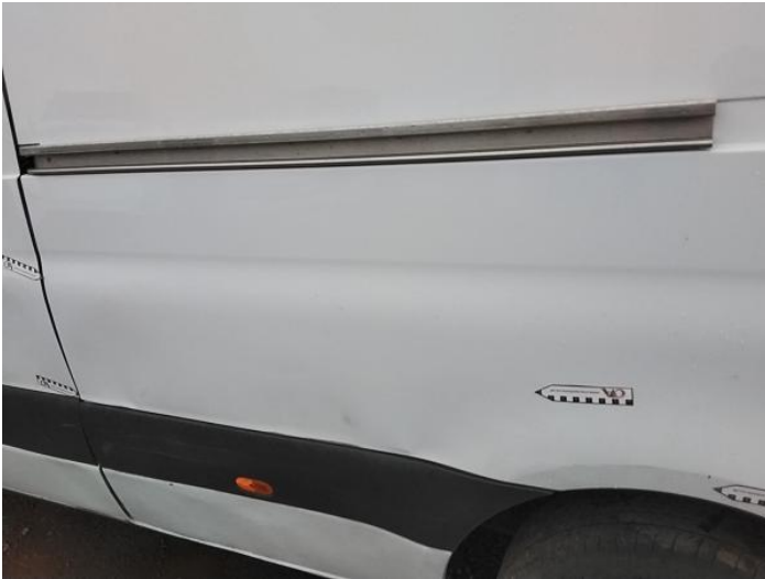
9: Qtr Panel nsr Dented Over 30mm
