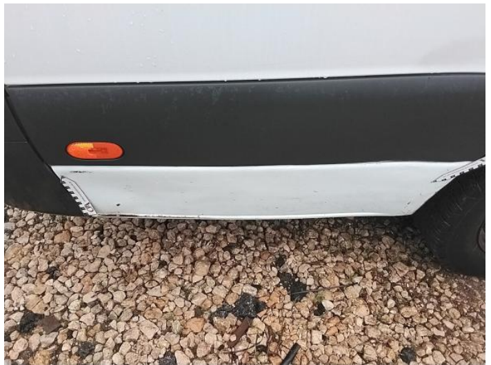
18: Qtr Panel osr Dented Over 30mm
