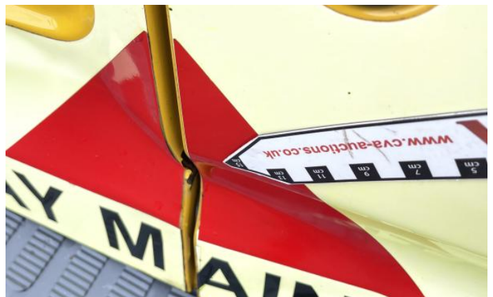
6: Qtr Panel osr Rusted Over 5mm
