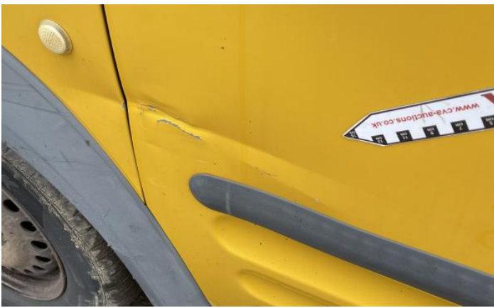
9: Door nsr Rusted Over 5mm
