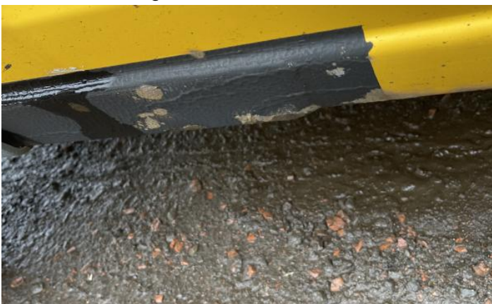
5: Door osf Dented With Paint Damage
