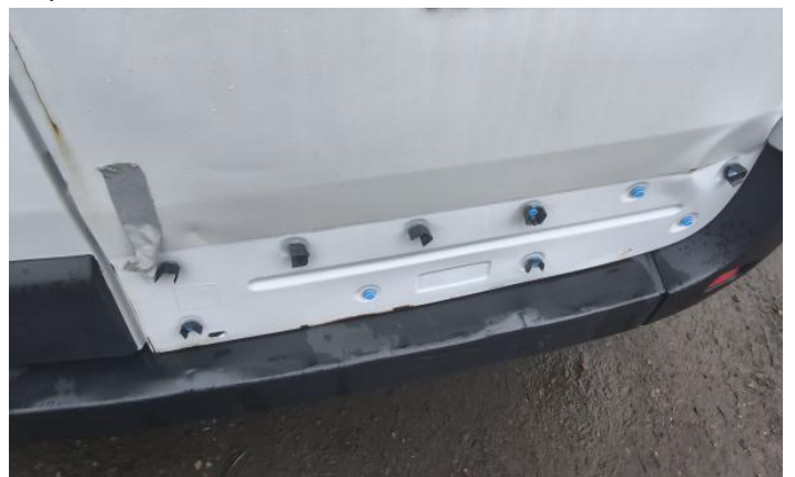
12: Aperture Seal nsr Missing Replace
