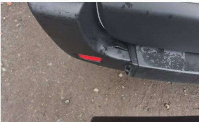
11: Qtr Panel nsr Dented With Paint Damage
