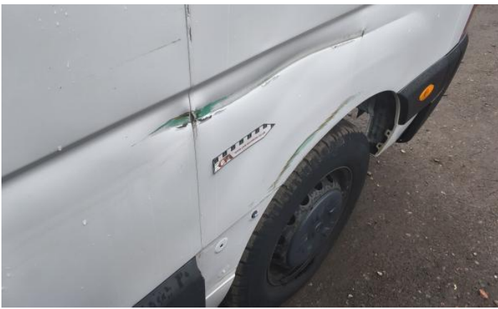
9: Qtr Panel Moulding ns Missing Replace
