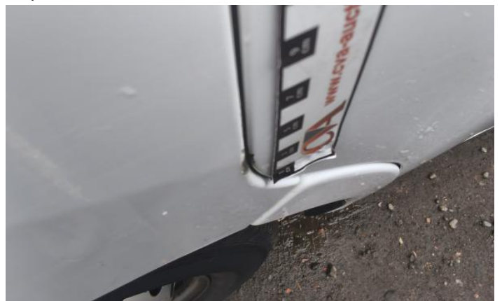
6: Bumper Front Moulding Broken Replace
