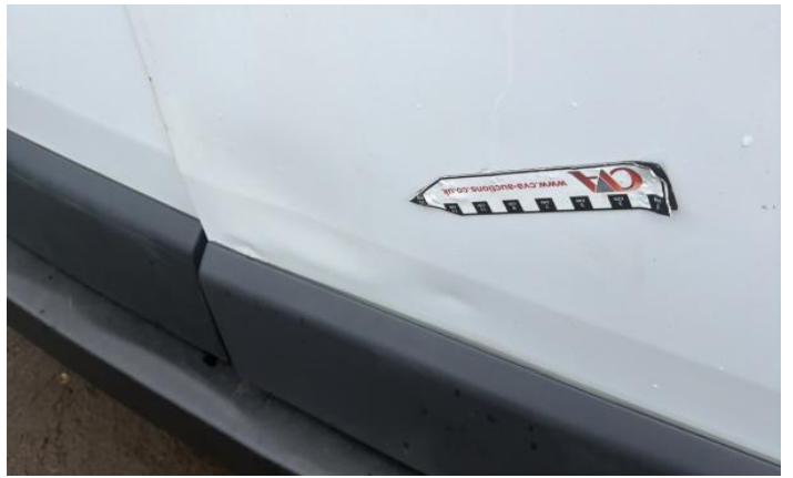
4: Door osf Dented With Paint Damage
