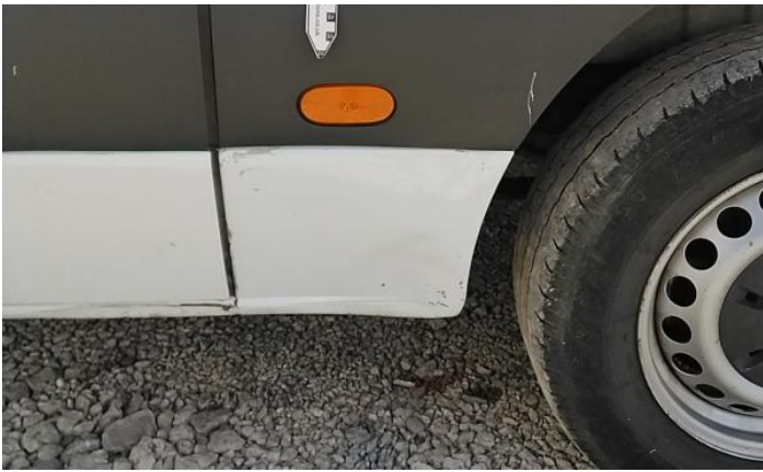
9: Sill ns Dented With Paint Damage
