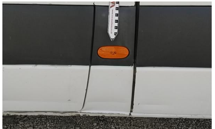
6: Wing nsf Dented With Paint Damage
