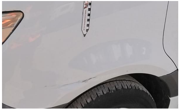
4: Bumper Front Moulding Scuffed (Unpainted) Over 100mm
