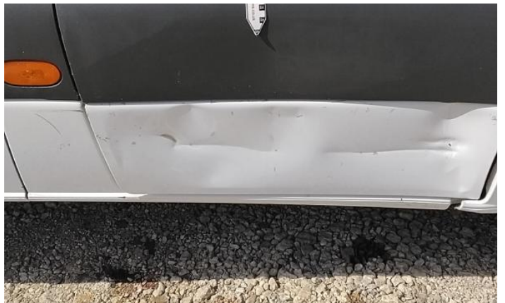
12: Sill ns Dented With Paint Damage
