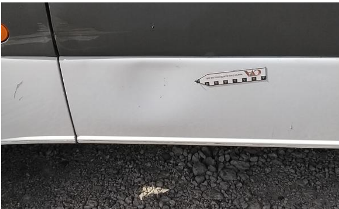
11: Qtr Panel nsr Dented Between 10mm + 30mm
