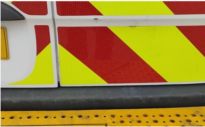
9: Door nsf Dented With Paint Damage
