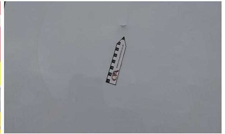
10: Door nsr Dented Over 30mm
