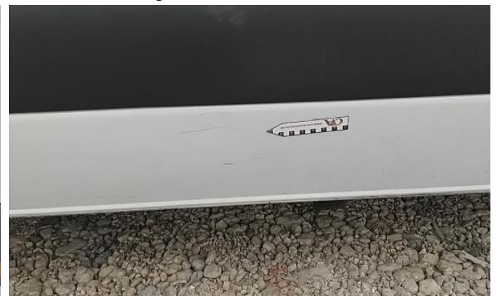
12: Door osr Dented With Paint Damage
