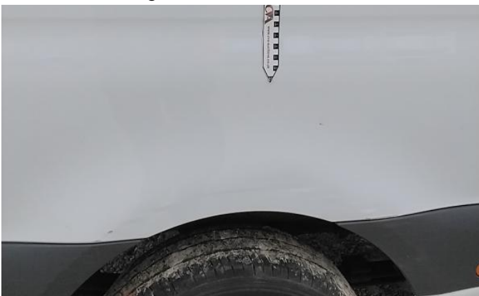
11: Door osr Dented With Paint Damage
