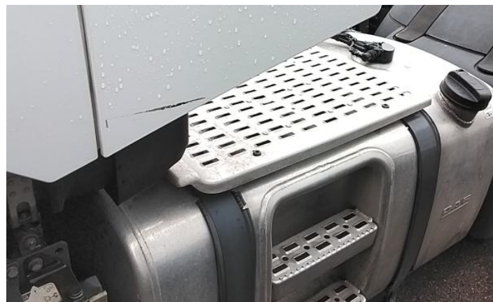
5: Door nsf Scratched Over 25mm Thru Paint
