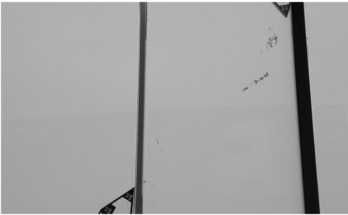
9: Panel Rear Scratched Over 25mm Thru Paint
