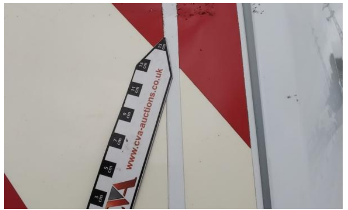
10: Qtr Panel nsr Dented Hail - Severe
