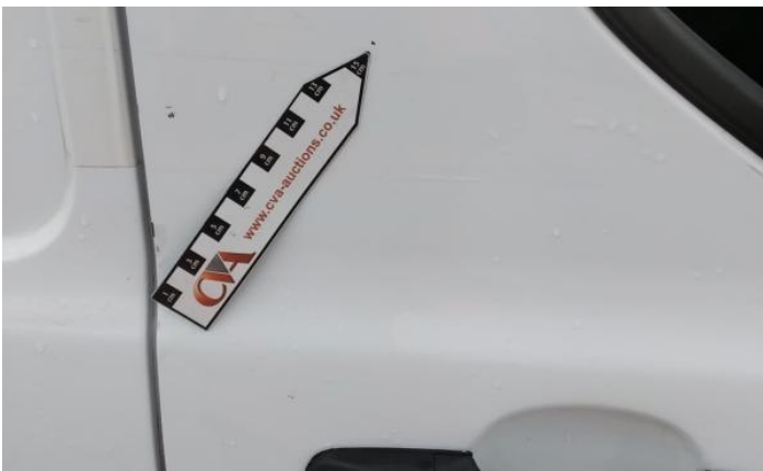
15: Qtr Panel osr Chipped Over 5mm
