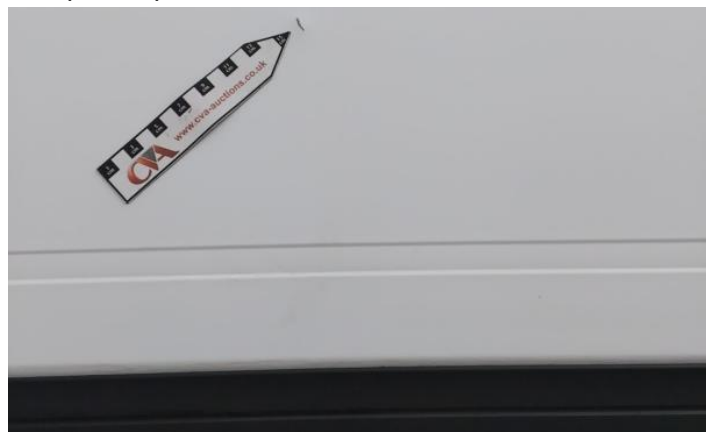
6: Door nsf Chipped Multiple Chips
