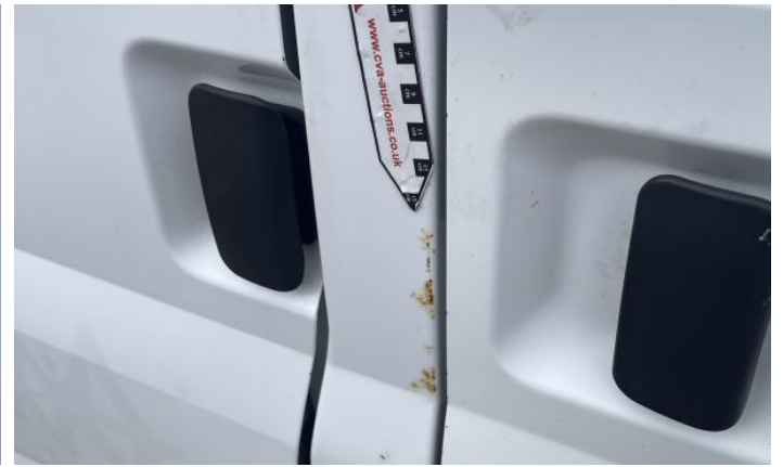
10: Qtr Panel nsr Rusted Over 5mm
