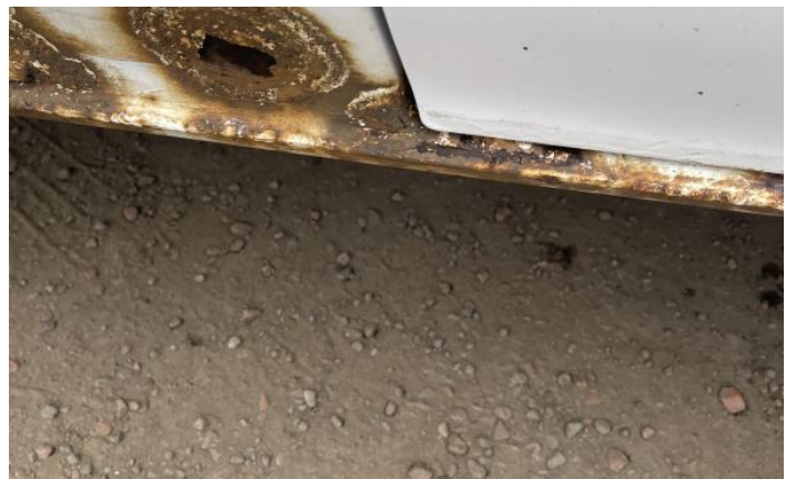
4: Door osf Rusted Over 5mm
