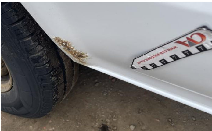
5: B Post os Rusted Over 5mm
