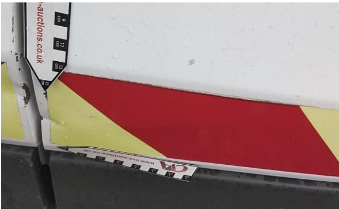
5: Bumper Rear Moulding Scuffed (Unpainted) Over 100mm
