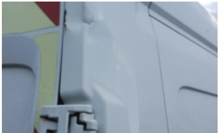
6: Door nsr Dented With Paint Damage
