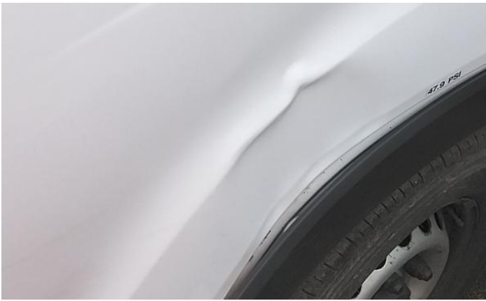
3: Panel Front Dented Between 10mm + 30mm
