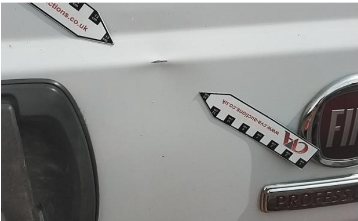
5: Qtr Panel nsr Dented Over 30mm
