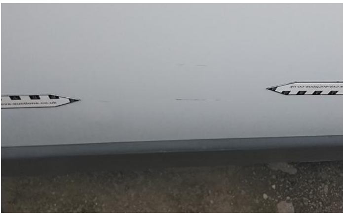
3: Bumper Front Scratched Over 100mm Thru Paint
