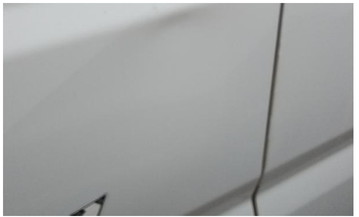
4: Door nsf Scratched Over 25mm Thru Paint
