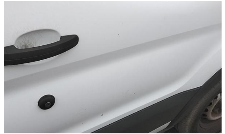
16: Qtr Panel osr Dented With Paint Damage
