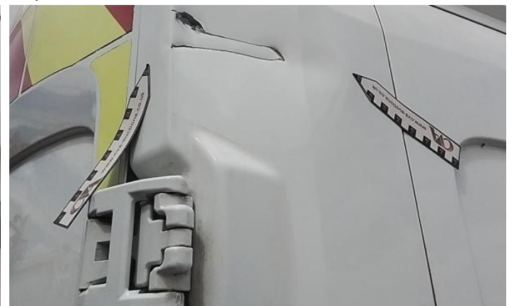
12: Bumper Rear Moulding Broken Replace
