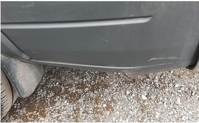
9: C Post ns Dented With Paint Damage
