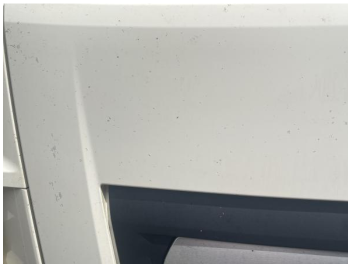
2: Bonnet Chipped Multiple Chips
