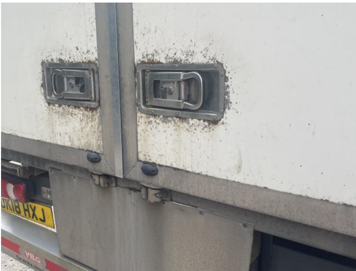
5: Tailgate Rusted Over 5mm
