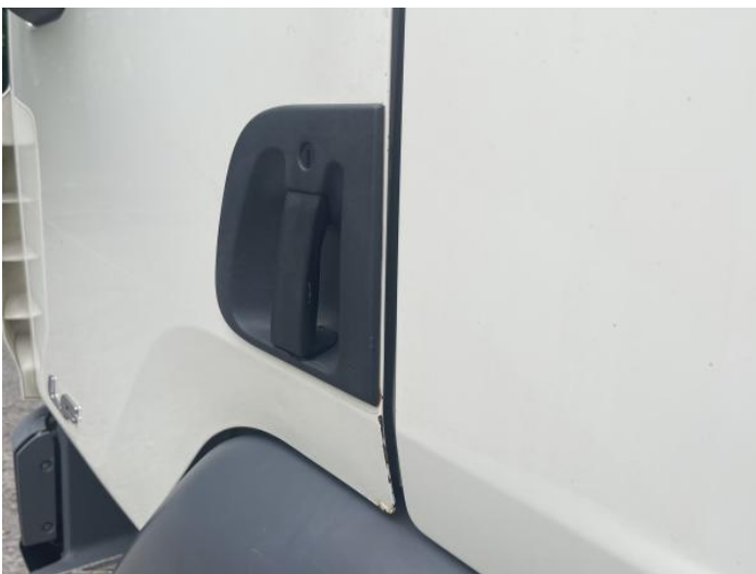
7: Door nsf Chipped Edge Chip
