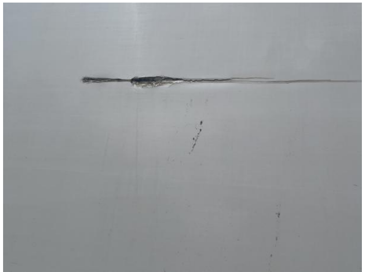
6: Qtr Panel nsr Hole Over 10mm
