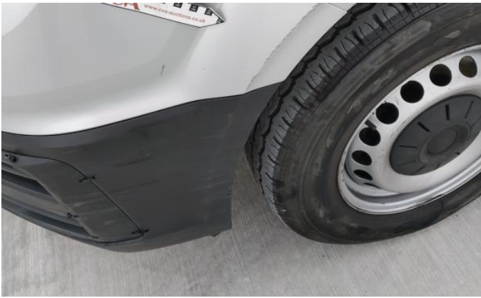
3: Bumper Front Insecure Action Required
