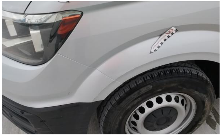
4: Bumper Front Scratched Over 100mm Thru Paint
