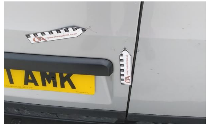
18: Bumper Rear Scratched Over 100mm Thru Paint
