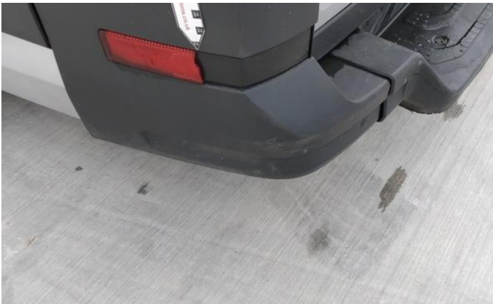
15: Qtr Panel nsr Chipped Over 5mm
