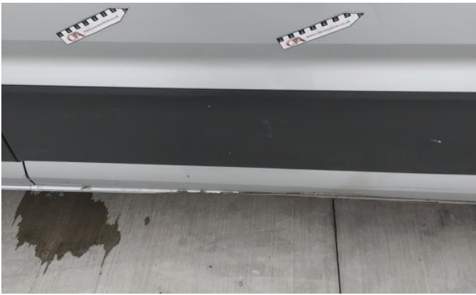
9: Door nsf Dented Over 30mm
