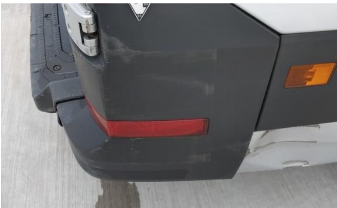
23: Panel Rear Dented Hail - Severe
