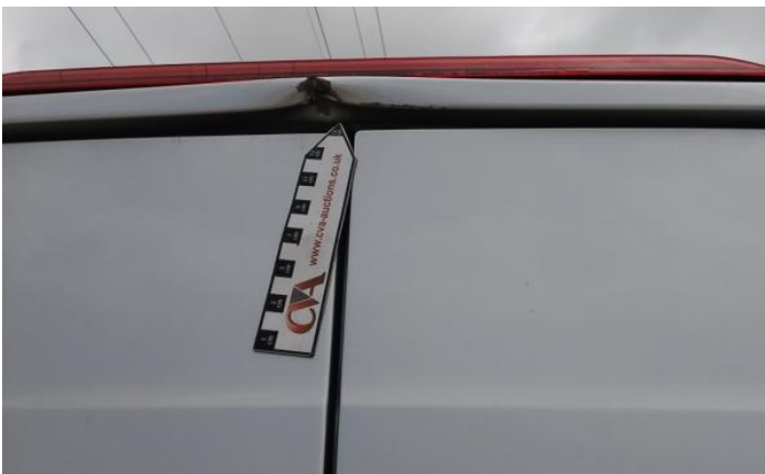
21: Door osr Chipped Over 5mm
