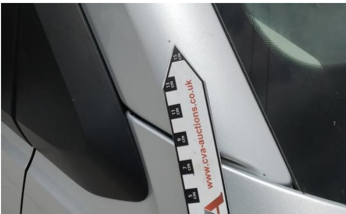
33: Door Mirror Assy osf Scratched (Painted) Over 25mm Thru Paint
