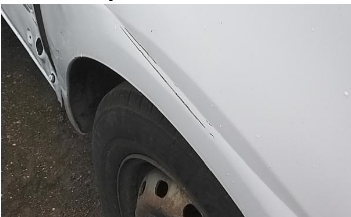
5: Wing nsf Dented With Paint Damage
