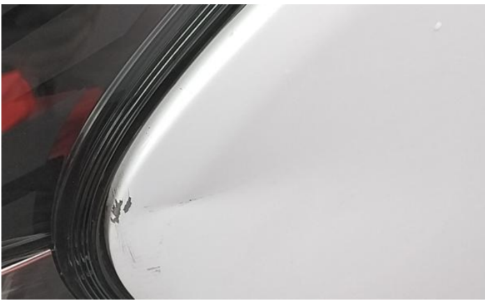
3: Bonnet Chipped Multiple Chips
