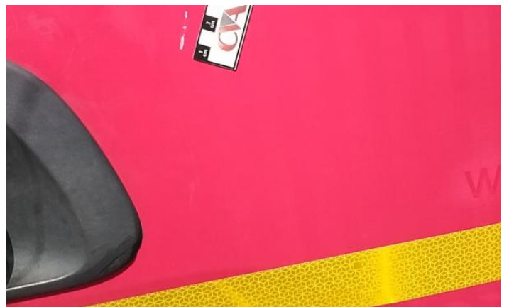
6: Qtr Panel osr Scratched Over 25mm Not Thru Paint
