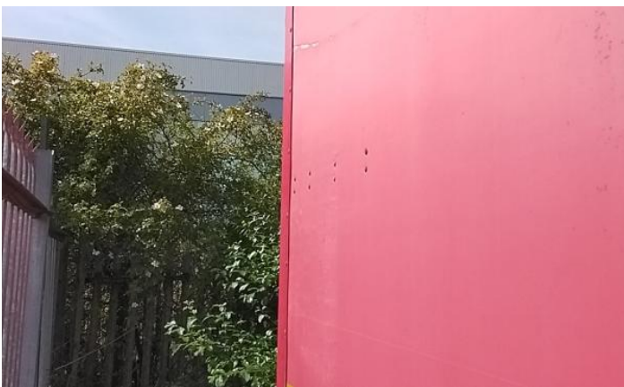
5: Wing nsf Scratched Over 25mm Thru Paint
