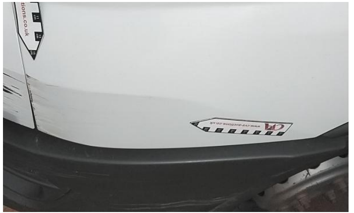
4: Bumper Front Dented With Paint Damage
