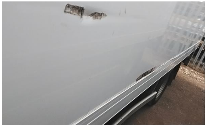
6: Wing nsf Scratched Over 25mm Thru Paint
