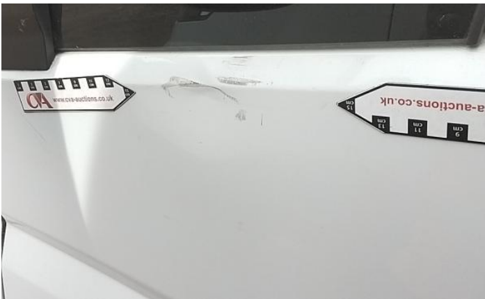
5: Panel Front Scratched Over 25mm Thru Paint
