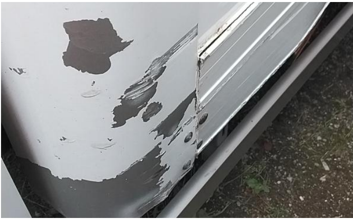
9: Panel Rear Scratched Over 25mm Thru Paint
