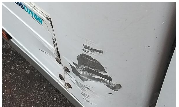
6: Bonnet Scratched Up To 25mm Thru Paint
