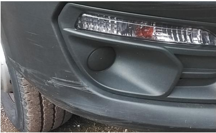
3: Bumper Front Dented Over 30% Of Panel
