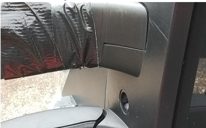
11: Panel Front Dented With Paint Damage
