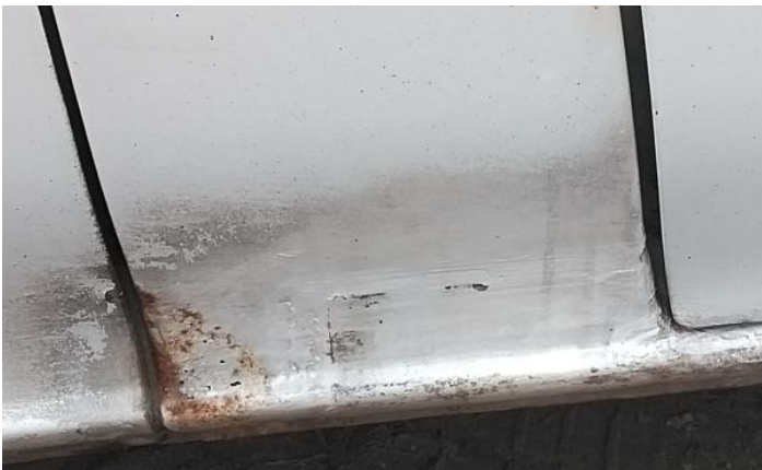
11: Panel Rear Rusted Over 5mm
