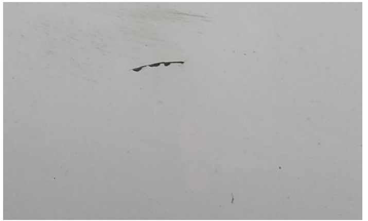
10: Bumper Rear Moulding Scuffed (Unpainted) Over 100mm
