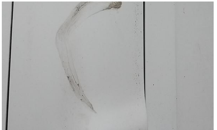
6: B Post ns Dented With Paint Damage
