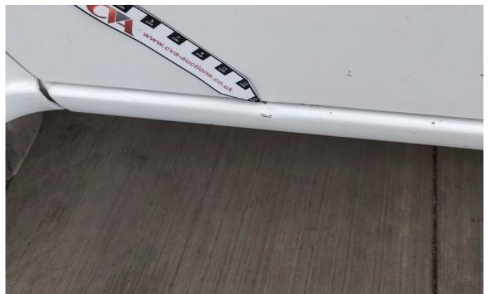
6: Wing nsf Dented Between 10mm + 30mm
