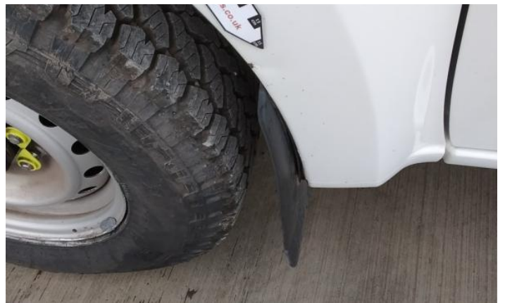
4: Bumper Front Moulding Missing Replace
