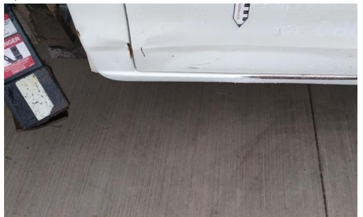
12: A Post os Rusted Up To 5mm
